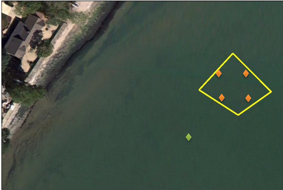
Figure 2 - Water quality monitoring stations at the study site. The yellow lines represent the barrier and perimeter of the treatment area. Orange diamonds represent monitoring stations within the treatment site and the green diamond represents the untreated control site monitoring location.
