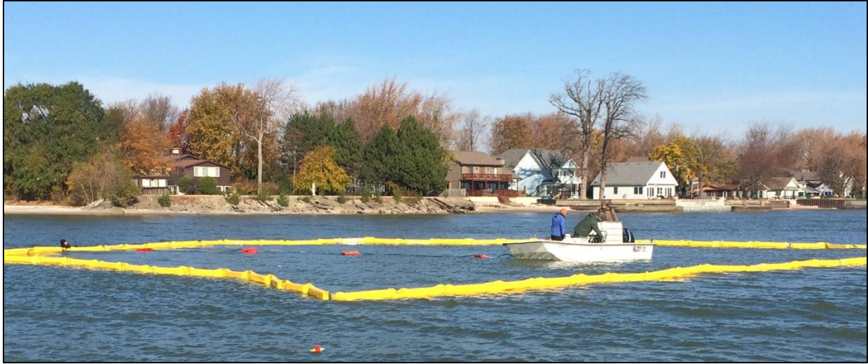
Figure 1 - Zequanox application within the treatment site. Drop hoses are located at each of the orange floats within the barrier. Photo credit: James Luoma, United States Geological Survey
