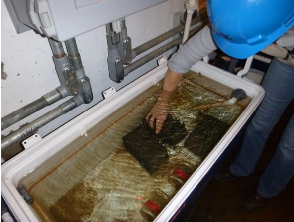
Figure 3. Monitoring Biobox. Visible in the biobox are three trays of settlement sample plates (one in the field scientist's hand) and two adult mussel containment tubes (of the three used in each biobox).
