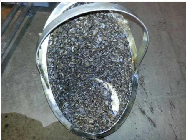
Figure 14. Strainer Basket that Required Cleanout on October 23, 2014. The baskets walls are covered in mussel shells in the image, while the small fish sits in the bottom of the cylindrical strainer basket. Credit Kevin Zito, Reclamation.
